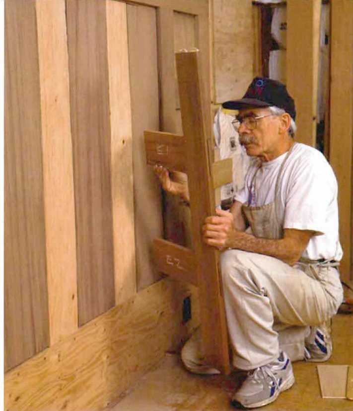
Cut the slots. With the help of a makeshift bench on a pair of sawhorses, the author plows grooves in the sides of the rails with a biscuit cutter. A clamped-on block backs up the cuts.
